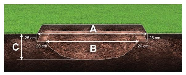
The hole should not accumulate water (in which case the drainage is necessary) and it should be possible to clean during maintenance.
