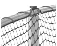
When the safety net is attached, the upper skirt should be placed on the frame of the net. Start placing the skirt at the door and sew the skirt together with the rope.
