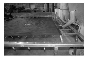
Place poles for the safety net. Poles need to be attached to the prepared sockets on the frame.
