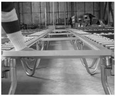
Place jumping mats with springs. Spread the jumping mat within the framework. Hook a short part of the spring to the jumping mat and the long side onto the frame. First place corner springs and continue with attaching every second spring. After these springs are attached, place the rest of the springs on the trampoline until all the springs are attached.
